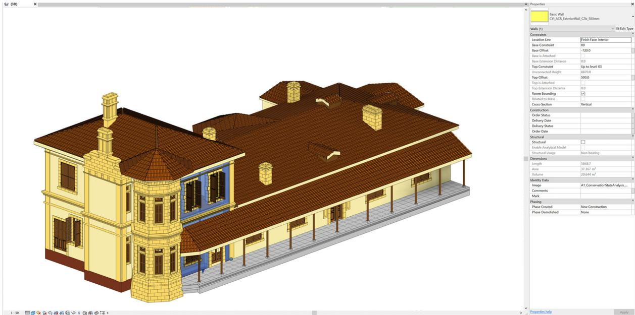
Fig. 10. Object selected to view its properties in the BIM model of the Cypriot pilot building.
