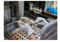
The production line starts with the manufacturing of the sand core by pressing silica sand into steel master moulds, depending on the type of piece to be manufactured.
