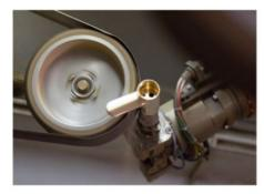
The degreased pieces continue to the grinding and polishing line, operations that are carried out before the chemical surface treatment.
