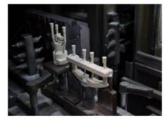
The sand cores continue to the casting line, where they are placed inside the moulds. Once the mould containing the sand core is closed, the casting of molten brass takes place, occupying the space between the sand core and the walls of the mould.
